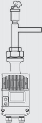
Fill system properly and vent. To vent the pump, this should be done as in chapter 7.3 Section IV. After this process, the pump can be set in the desired control mode.
